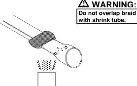
4 Slide a 13mm (0.5") diameter, 51mm (2") length shrink tube over the heater cable leaving approximately 25mm (1") of shrink tube past the heater cable. Shrink with heat gun until completely shrunk.
